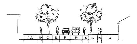
**Figure 7b.** Schematic sketch of a typical sub-collector street cross-section. Table 1 lists the recommended dimensions of each component: A) building setback from street right-of-way; B) walkway; C) planting area; E) bicycle lane; F) travel lane.
