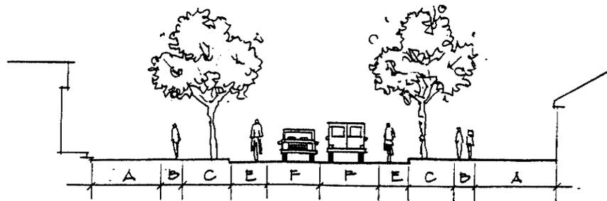
**Figure 7b.** Schematic sketch of a typical sub-collector street cross-section. Table 1 lists the recommended dimensions of each component: A) building setback from street right-of-way; B) walkway; C) planting area; E) bicycle lane; F) travel lane.
