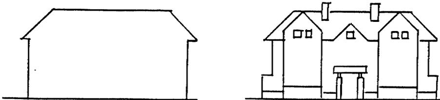
**Figure 11.** Schematic elevation sketches of two multi-storied buildings with equal heights and widths. Architectural details such as porches, windows, and roof dormers articulate a building's facade (right) which enhances visual quality and contributes to a human-scaled development.
