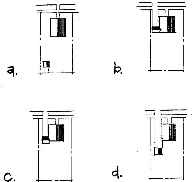
**Figure 12.** Plan-view diagrams of four alternative garage locations on a single-family housing lot: a) detached garage is accessed from an alley; b and c) attached garage is accessed from the local street, d) detached garage, behind the house, is accessed from the local street.
