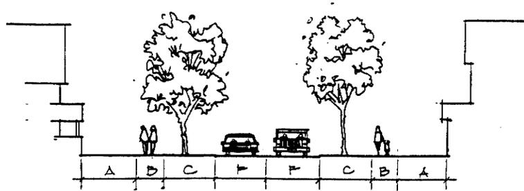
**Figure 7a.** Schematic sketch of a typical local street cross-section. Table 1 lists the recommended dimensions of each component: A) building setback from street right-of-way; B) walkway; C) planting area; F) travel lane.
