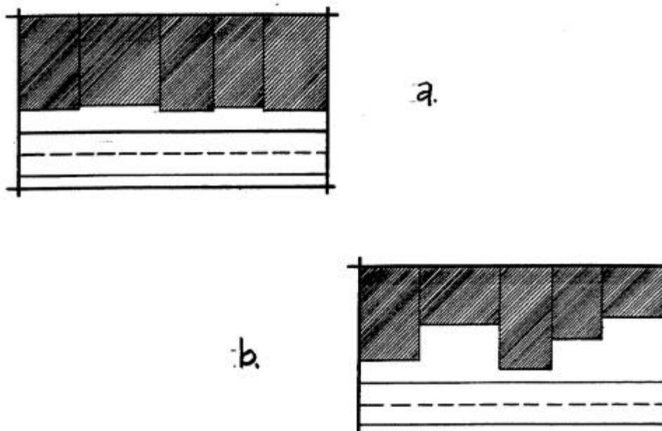
**Figure 5.** Plan-view diagrams showing two alternatives for building setbacks from the street right-of-way in mixed-use areas. Relatively uniform setbacks (a) are preferable to widely varying building setbacks (b).
