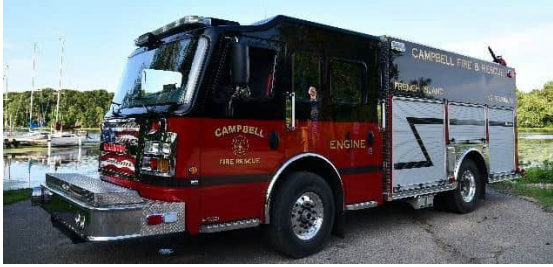
Engine 1 - 1500 GPM, 1000 gallons
