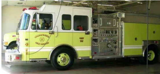
Engine 1 - 1500 GPM, 1000 gallons
