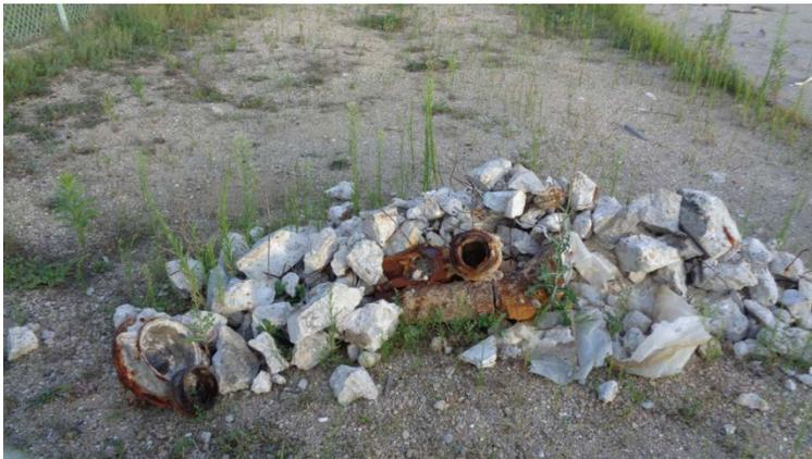
The concrete, plastic, and rusty pipe in the referenced picture is located in an area which had no detectable concentrations of PCBs in soil from the Phase II ESA sampling event. The material indicates no observable staining other than from contact with the exterior of the rusted pipe embedded in the concrete. The material will be disposed along with other demolition debris from the project at an appropriate offsite facility.
